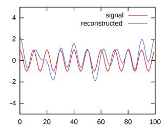
The filtered signal shown in blue, along with the original signal in red.
