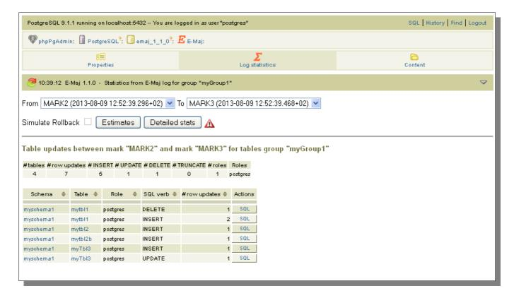
Figure 9 – Detailed statistics about updates recorded between two marks
