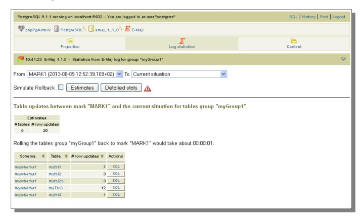
Figure 10 – Result of the rollback simulation, with the estimated number of updates concerned for each table.
